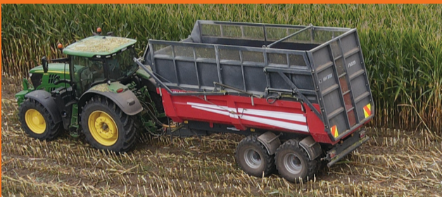
HM 3100 Silage/Dirt Trailer Two trailers in one, 31.0m 3 Silage, 12.0m 3 dirt, Leaf-spring drawbar, Fast bin removal
