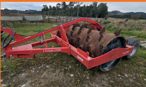
TITAN LV300 Spiked Aerator 2021, 3m working width, Hardox aerating blades
