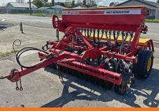
**DUNCAN Renovator Mk3** Farmer Owned, 6" row spacing, Tidy machine, Easy to calibrate, Easy to run
