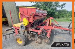
**DUNCAN Renovator Mrk 3 Direct Drill** 19 run, 3.0m sowing width, Twin box, Covering harrows, Hydraulic opening disc
