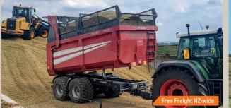
HM 3000 SILAGE/GRAIN TRAILER - EX DEMO 30m<sup>3</sup> capacity (able to be towed with as low as 130Hp), 650mm wide tyres, 4-wheel hydraulic brakes, Watertight door seal
